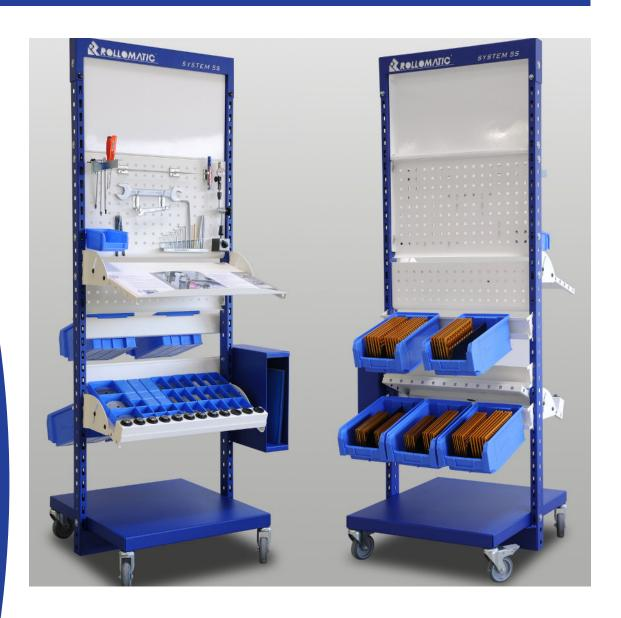
The Rollomatic 5S mobile shadow board is designed to store and organize all essential hand tools, accessories and documentations necessary for the efficient operation of your grinding machine.
