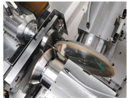
Top view of the pinch/peel grinding process on the ShapeSmart NP50
