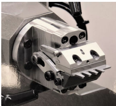
Clamping of a woodworking profile blade
