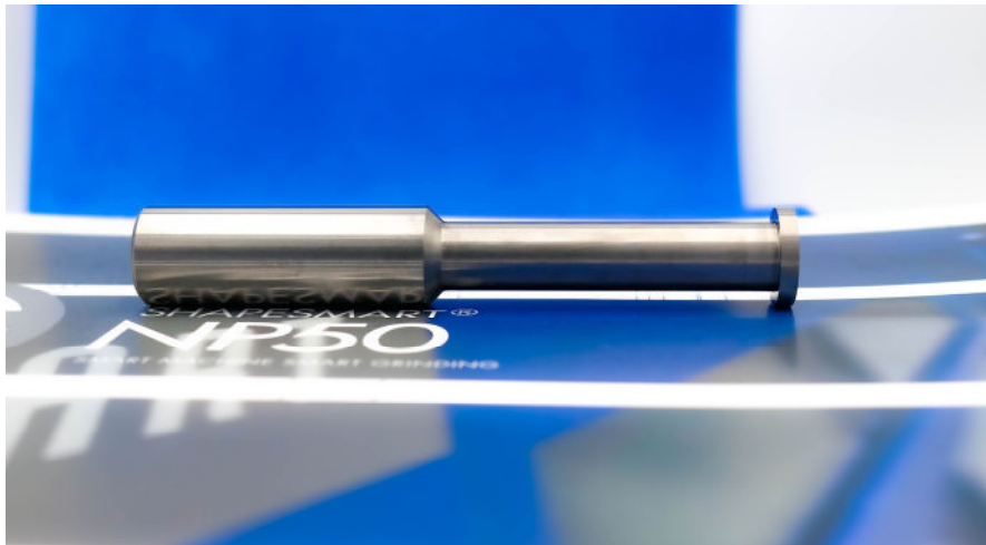
T-slot blank in solid carbide ground by the ShapeSmart® NP50 in one set-up
